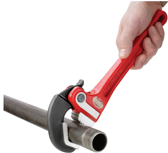
Figure 5 – Using a RapidGrip Wrench
