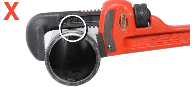
Figure 4 – Wrench Too Small For Work Piece, Hook Shank Touching Work Piece.
